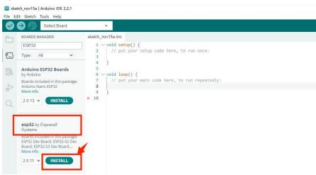
6. Once installation is complete, close the Arduino IDE program and reopen it. When you go to Tools > Board. You will see the esp32 board appear.
