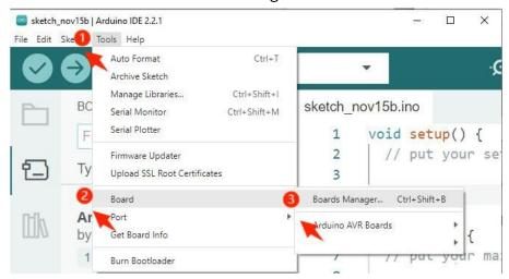
5. Search for "ESP32" in the BOARDS MANAGER's search bar and install "esp32 by Espressif Systems."
