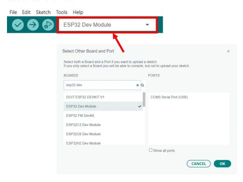
Use the "Verify" function to compile the code to see if there are any issues. Then use "Upload" to send the program code to the ESP32 control board in the rover. Debug can be used if errors are encountered.
