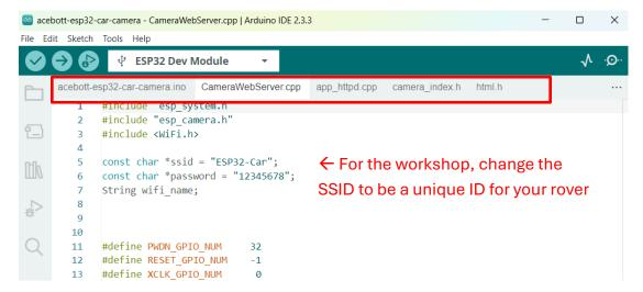
5. Make sure to select the "ESP32 Dev Module" and correct COM port for your computer.
