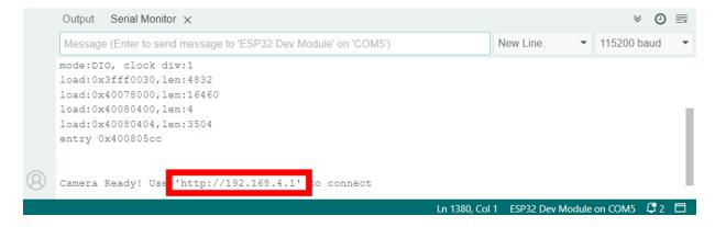
9. On your computer, go to your WiFi settings and find the SSID for your rover. Connect with the password (12345678 by default) and go to the indicated web address in a web browser. Your WiFi should be connected, and will show that there is no internet (this is the correct setup).
