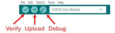
Arduino IDE will show progress in the "Output" section and will take some time to compile code, connect to the board, and upload program.
