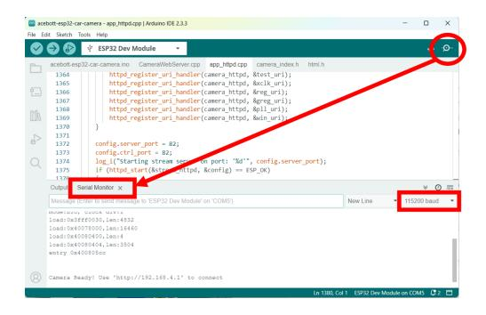
8. Then, click the white "reset" button on the camera module, next to the USB cable connection (see image in step #1). After clicking the button, data should appear in the Arduino IDE Serial Monitor. Note the http address listed to connect to the camera via a web page.
