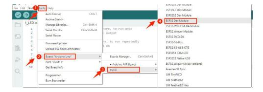
Lumi said happily: "Very good! Next, connect the ESP32 board to your computer using the USB cable, and then select the corresponding port number on the Arduino IDE, and finally upload the program to the board."
